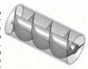
second can pass through each screw, generating a total of up to 100kW of electrical power. Environment Agency records for the Thames go back up to 70 years, giving confidence in the expected long term output.
